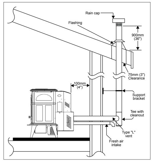
Figure 14: Outside Vertical Installation.
